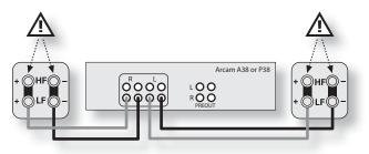
An A38 or P38 connected to speakers using single wiring
