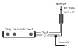
The A38 can also provide a +12V trigger output to control devices such as the power amplifier in Zone 2. The +12V trigger is active when the unit is 'On'.
